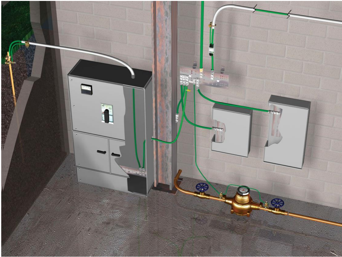
Figure 3: Grounding and Bonding at the Service Entrance
