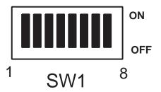
DIP switches are for assigning an address to the RAXN-LCD. Binary addresses 33 to 39 are available with the least significant bit being switch SW1-1 on the left and the most significant bit being SW1-6. The ON setting is active binary. DIP switches SW1-7 and SW1-8 are not used.
