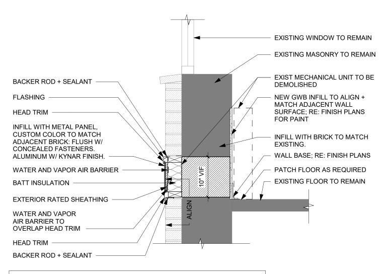
INVESTIGATIVE DEMOLITION REQUIRED TO CONFIRM/DETERMINE THE MAKEUP OF THE EXISTING WALL. INFILLED AREAS ARE TO MATCH EXISTING, INCLUDING WATERPROOFING, FLASHING + THERMAL INSULATION.
