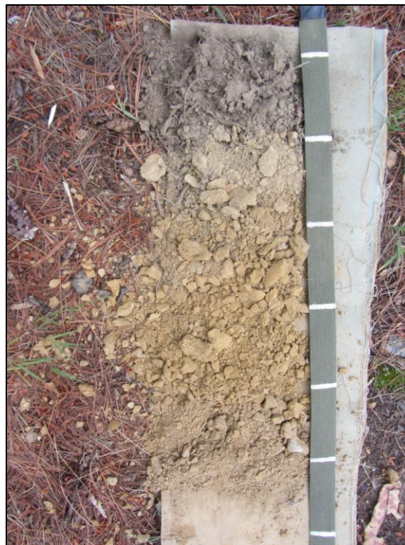
Figure 1. At the location of Boring 2 a nearly intact soil is formed in a mantle of loess atop a buried paleosol surface at the depth of 41 cm.
