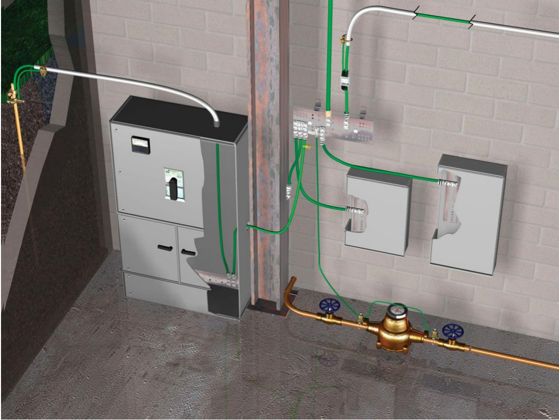
Figure 3: Grounding and Bonding at the Service Entrance
