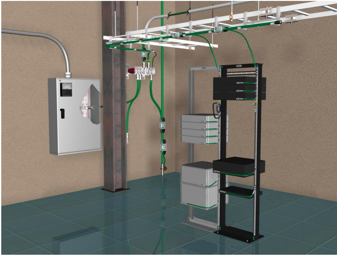
Figure 5: Grounding and Bonding in Telecommunications Room
