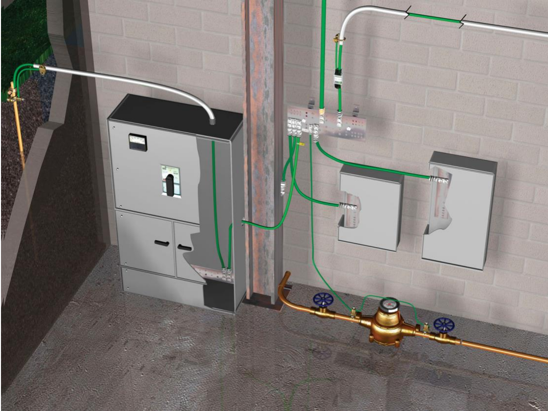
Figure 3: Grounding and Bonding at the Service Entrance
