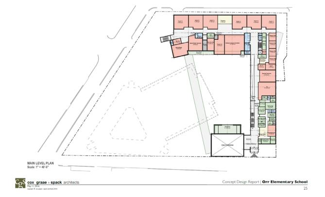
The "dashed" line represents the existing building and when combined with the proposed new building nearly all of the project site will be occupied. The "north-south" connector that bi-sects the existing building will be constructed as part of the second phase of the project (i.e. the demolition and site work).
