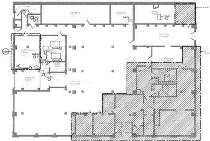
2 ELECTRICAL FIRST FLOOR DEMOLITION PLAN DATE: 10/1/19
