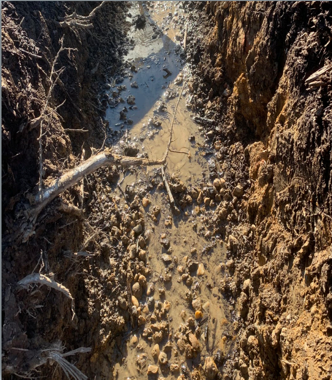
Groundwater visible and flowing in the trench from the higher elevations at southwest to the field to the north.
