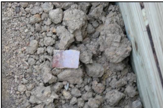
Photographs of construction debris and soil medium below lawn and planting areas.
