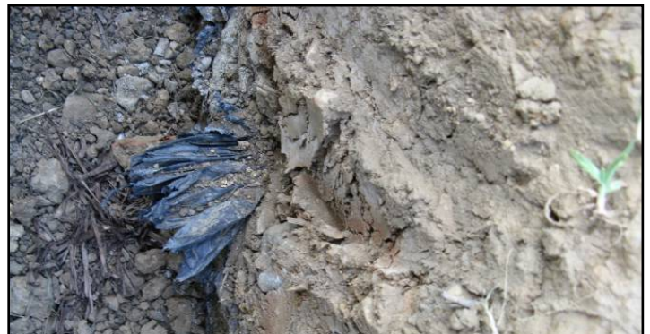
Photographs of construction debris and soil medium below lawn and planting areas.
