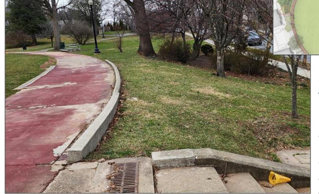
Proposed location for a new bioretention on the southeast side that of the field is tied into all the field underdrains; removal of (2) trees and the installation of (1) new honey Locust tree.
