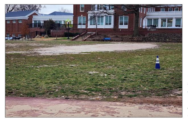
Existing conditions highlighting the bare spot on the field from compaction and lack of drainage.
