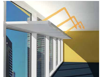
HORIZONTAL SHADING AND LIGHT SHELF AT SOUTH FACADE
