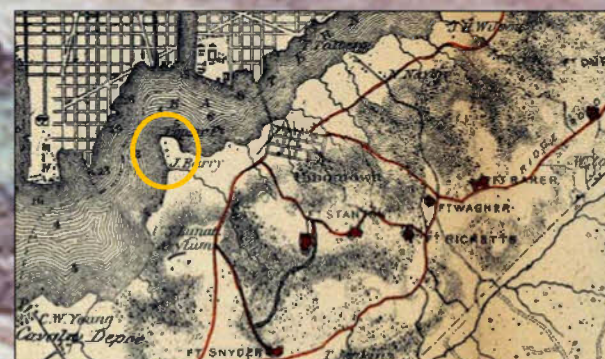
1865 "Civil War Defenses of Northern Virginia" The original shoreline of the Anacostia River before landfilling is shown. Note how much smaller Poplar Point (in the circle) is than today, and how many streams drained into the river. The string of forts, in dark red, were linked by military roads. Source: Library of Congress gwb01c040011
