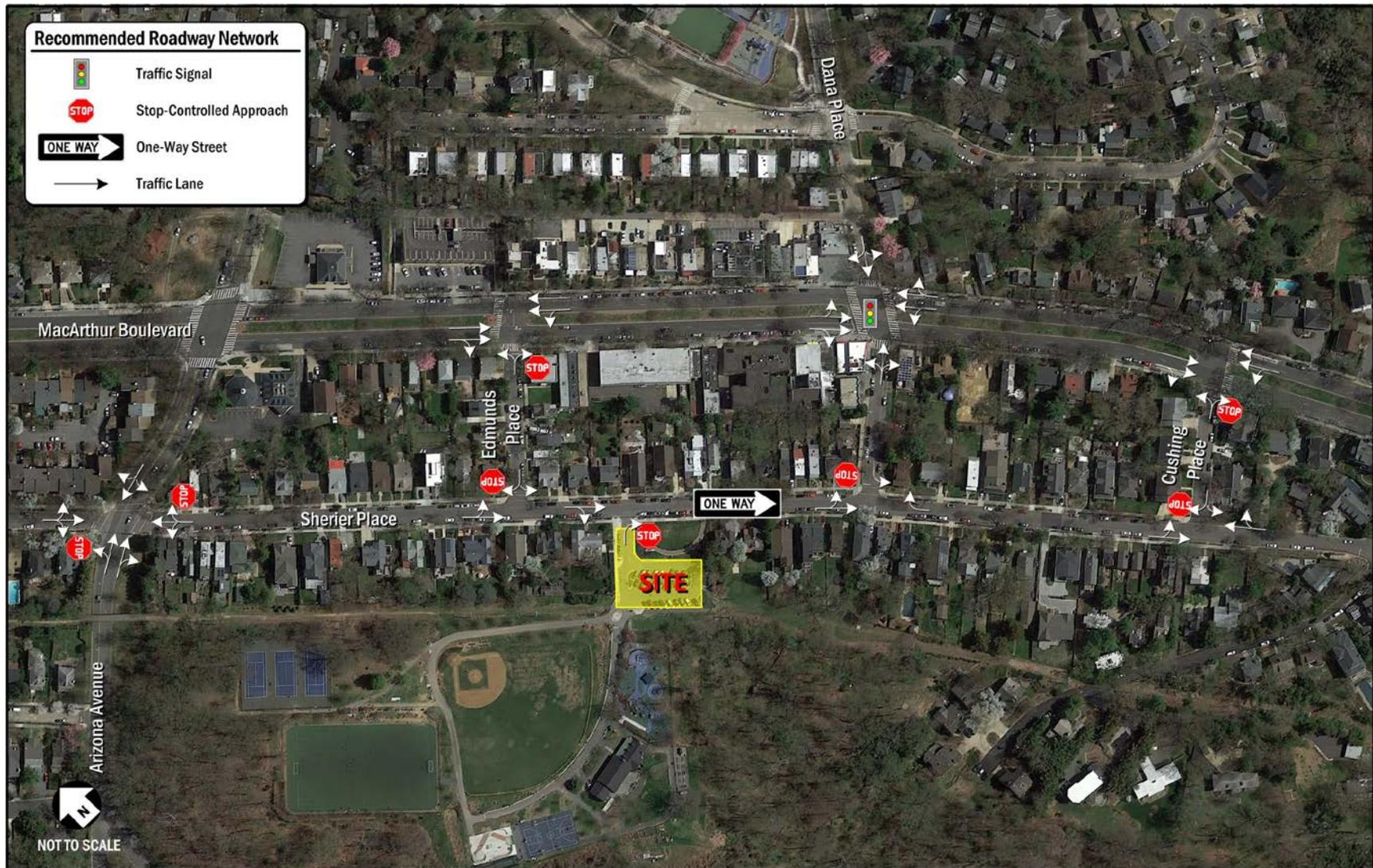
Figure 7: Modified Lane Use and Traffic Control
